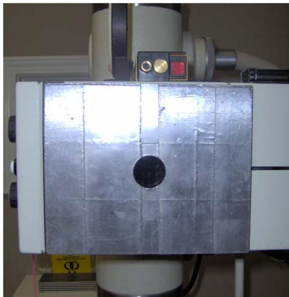
**Figure 5: Vertex filter affixed to collimator**
